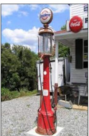
graduated glass cylinder and then, by gravity, the gas was dispensed into the car.
